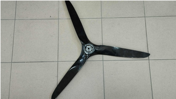
Fig. 5. View of propeller mount breakage due to overspeed overload Source: Own study
