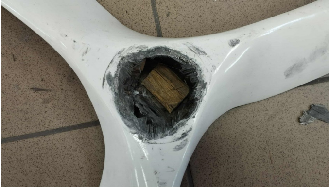
Fig. 4. View of damaged propeller mount – 3-blade composite propeller Source: Own study
