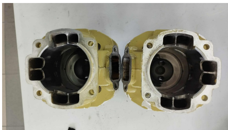
Fig. 13. Damaged inner part of the cylinder smoother due to overheating of the head
