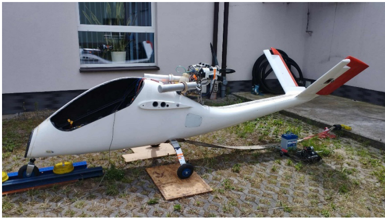
Fig. 2. Test bench using a real OSA 3 aircraft with an engine mounted on the fuselage Source: Own study
