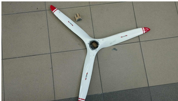
Fig. 3. View of damaged propeller due to excessive angular vibrations
