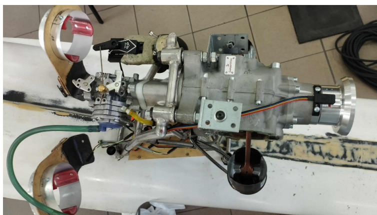
Fig. 9. View of the internal combustion engine block layout with the cylinders removed after the engine seizes
