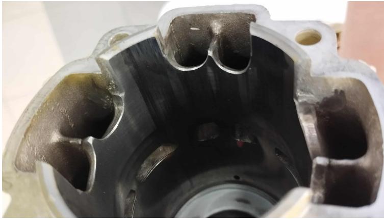
Fig. 10. Damage to the cylinder smoothing due to the disappearance of the fuel-oil film
