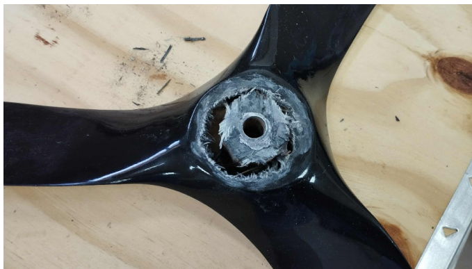
Fig. 6. View of the damage to the 3-blade carbon fibre composite propeller mount Source: Own study
