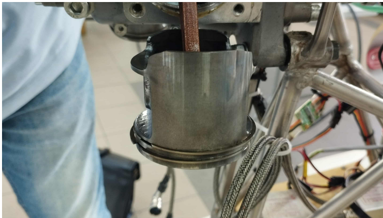
Fig. 11. Damage to the piston side surface due to sudden resonance vibrations of the drivetrain
