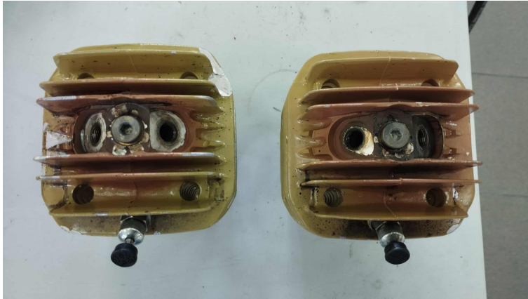
Fig. 14. View of overheated heads of a small two-stroke aircraft engine
