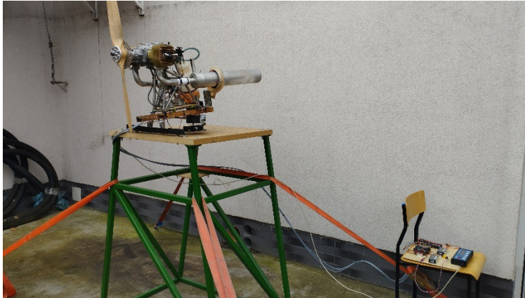
Fig. 1. Frame test bench designed for testing piston internal combustion engines in a frame system Source: Own study
