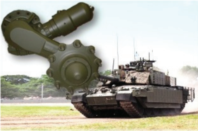
Fig. 3. Challenger tank hydropneumatic spring
