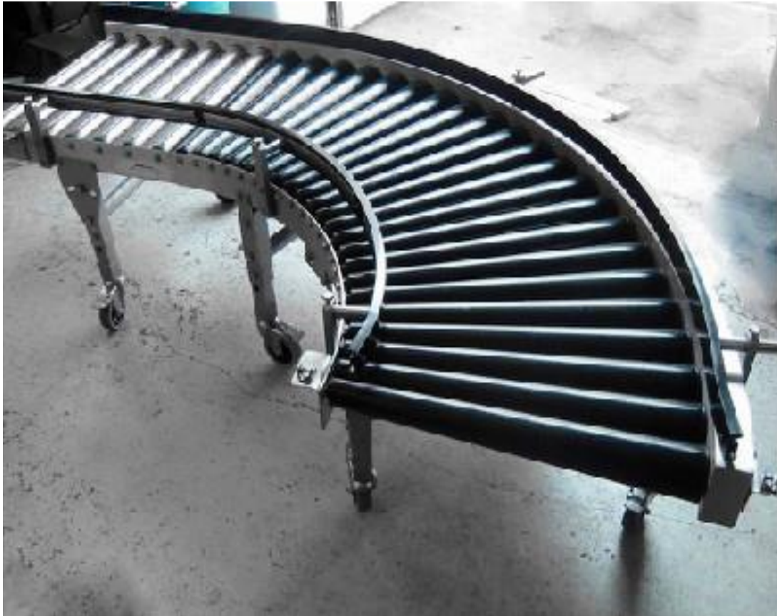
Fig. 2. Gravity conveyor, moving commodities by using the g – force.
